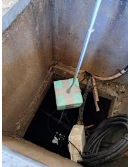
Figure 2.8: Sinking the sensor along with a floating buoy to keep the pending rope under the water level and the sensor inside the water.
