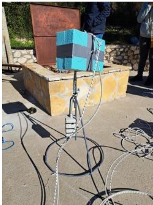
Figure 2.14: The CsI (TI) detector no. 3 - Sensor unit S006 and the dangling system used for supporting the sensor.
