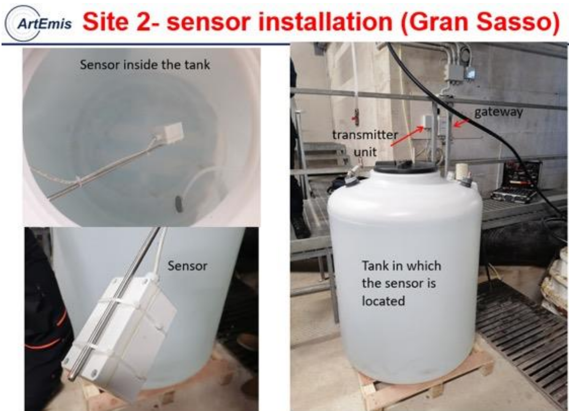
Figure 3.8: Installation logistics of the site 2 (NE Gran Sasso groundwater intake tunnels): tank in which is located the sensor prototype.
