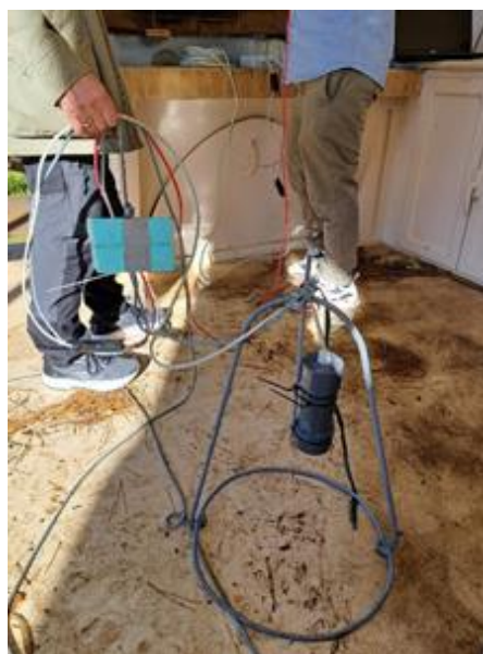
Figure 2.7: The Scionix detector no. 3 - Sensor unit S003 V3.1 and the dangling system for supporting the sensor.
