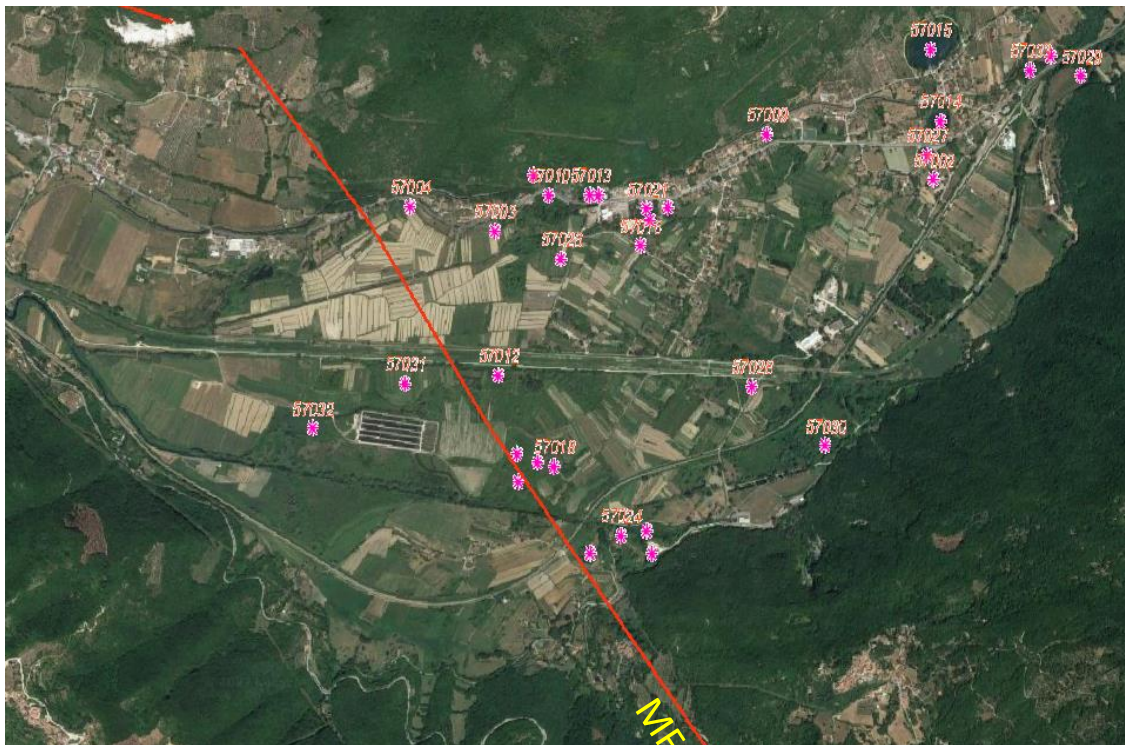
Figure 2.7: The hydrothermal area of Cotilia spa (30 km west to L’Aquila) in which sinkholes by ISPRA database ( http://sgi2.isprambiente.it/arcgis/services/servizi/sinkhole/MapServer/WmsServer ) and seismicogenic faults by ITHACA database ( http://sgi.isprambiente.it/ithaca/viewer/index.html ) are reported. Note the sinkholes aligned along the seismicogenic fault which cross the Velino R. plain (Miccianni fault Auct.: MF)
