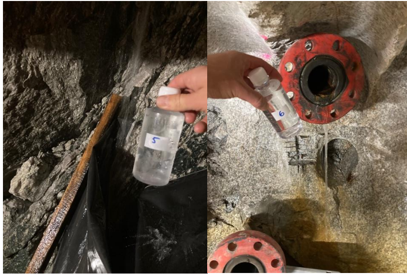
Figure 4.3 Example of water sampling from a) a fracture zone and b) a borehole (Photos: M. Strupler)
